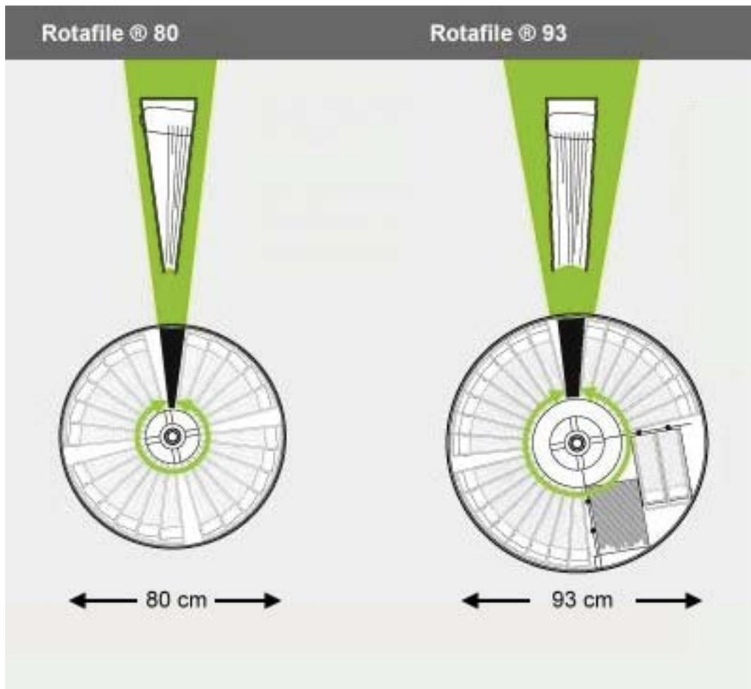
The **80 cm** rotary files can hold a maximum **24 wedge-shaped binders** per level.
